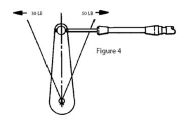
The output motion of the workend of the cable is essentially the same as the input motion. For example, a 3" pushing movement at the input end will result in a 3" pushing movement (less backlash) at the output end. If a differential between input/output and/or direction of movement is desired, it must be accommodated in the design of the lever and attaching point at the workend. See Figure 6.
