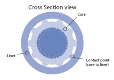
TFXtreme's unique design incorporates a splined core to achieve the "impossible". Ridges of the core allow a close fit with the cable's inner liner, but with minimum contact, so the core glides back and forth smoothly. The result – easy movement and minimum lost motion.
